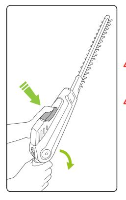
Firmly grip the head of the trimmer and press and hold the green button. Rotate the head to your chosen angle. Release the button to lock the head in position.
