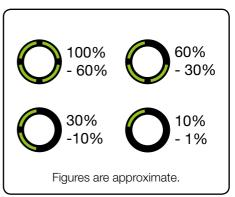
Press the button to check how much charge The number of lit LEDs shows the charge. there is in the battery.
