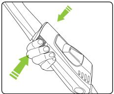
Press the green buttons on either side of the trimmer head.
