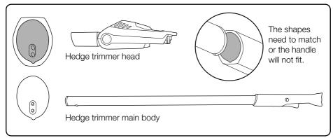
When inserting the body into the hedge trimmer head, ensure the body is the right way up. The shapes need to match or the handle will not fit.
