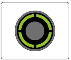
When the battery is fully charged the LEDs will stop pulsing and remain green in colour.
