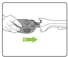
Insert the battery, which will click once fully inserted.
