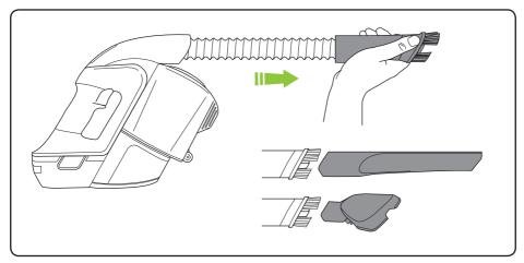
An extendable hose is built into your Multi. Pull the black tube forwards to release it. Use the extendable hose with any of the accessories for hard to reach areas.
