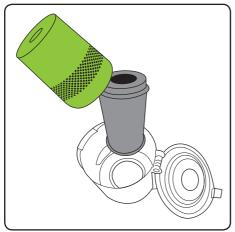
If the filter light comes on when the bin is not full, wash the filter. The filter is inside the green filter case which just pulls out of the Multi's bin.
