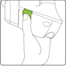
Press the green buttons and pull to remove the battery. The battery can be charged on or off the main unit. If you want to buy a spare battery go to **www.gtechonline. co.uk** or call **01905 345891**
