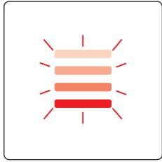
When the lights rapidly cycle red, recharge the battery.
