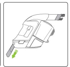
The brush can be used for dusting. The crevice tool is stored inside the handle.
