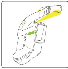
Press the trigger lightly to turn on the headlights and see the battery level. Press the trigger firmly to vacuum.
