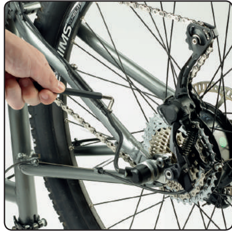
Using the tool redo the cable guide which holds the hub connector cable in place.
