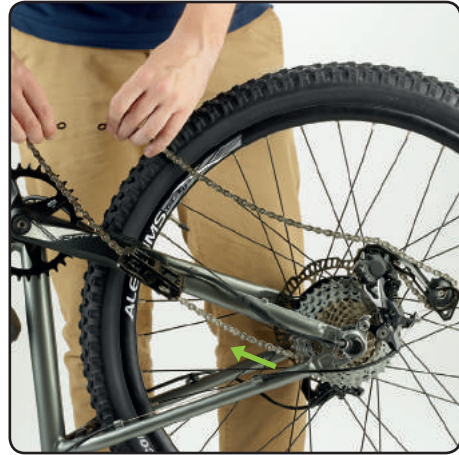
Pull the two ends together, making sure the one end goes through the frame of the bike.
