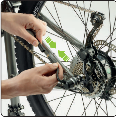
Reconnect the hub connector cable.
