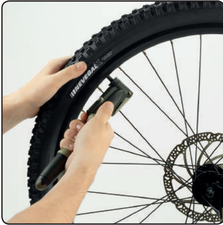
Release the thumb lock by pushing the lever back down.
