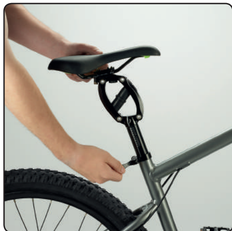
Pull back the quick-release lever.
