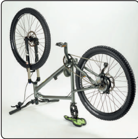
Adjust the saddle so that it is at its lowest position. Turn the bike upside down and place on a soft surface.
