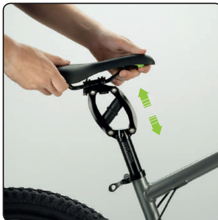
Adjust the saddle to the correct height for you, making sure that the minimum mark is not above the seat tube.
