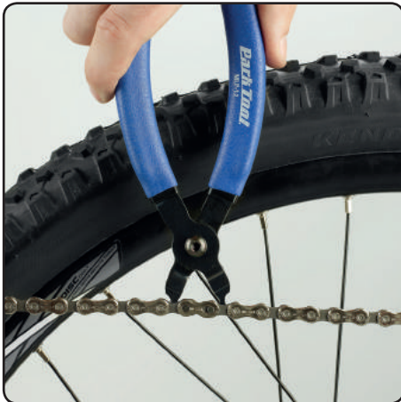
Insert the master link pliers into the master link.
