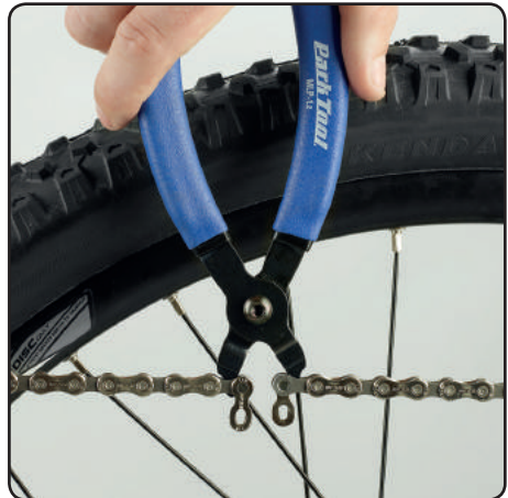
Squeeze in the handles. This will detach the master link and it can now be removed.
