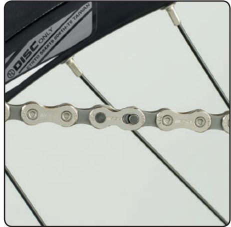
Locate the master link in the chain. The master link is different to all the other links as it has black pins rather than chrome.
