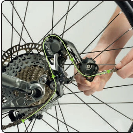
Feed the new chain through the derailleur.
