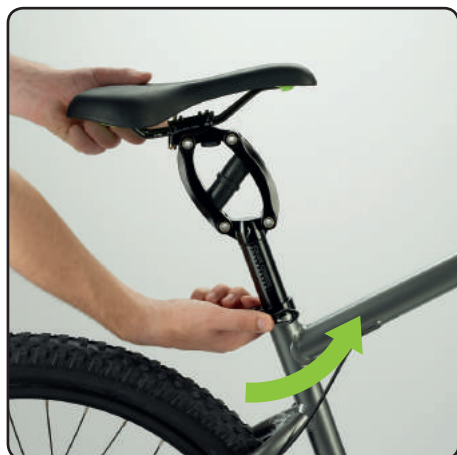
Close the quick-release by firmly pushing on the quick-release lever, so that it lies flat against the frame. If necessary tighten the adjusting nut, until you need to use the palm of your hand to close the quick-release lever.
