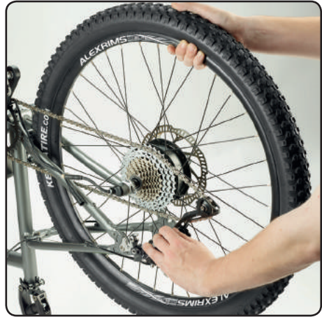
Whilst still holding back the derailleur, pull the wheel up to remove. You may have to move the chain out of the way.
