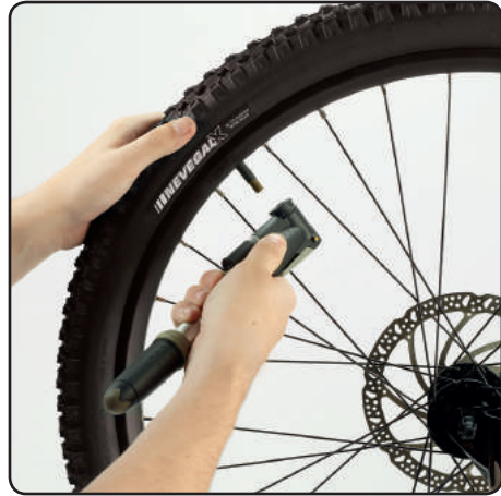
Remove pump nozzle from the valve stem.
