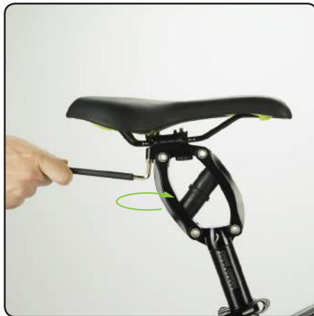
Turn the screw clockwise to tighten it to your preferred setting.
