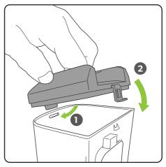
To refit the lid locate the tab into the slot in the tank then close to the latch.
