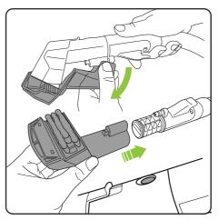
Remove the self-cleaning cover from the cleaning head. Push the cleaning head onto the end of the hose until it clicks into place. Ensure the button is engaged into the hole.
