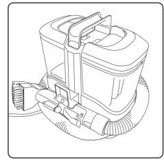
Wrap the hose around the unit and clip the cleaning head into the holder.
