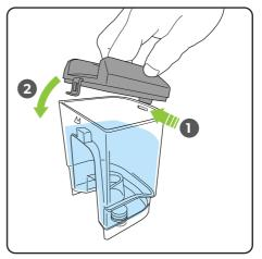
To refit the lid locate the tab into the slot in the tank then push the lid down until it clicks shut.
