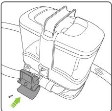
Fit the brush holder to the unit and secure with the screw.
