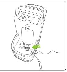
Remove the waste water tank Use a suitable tool to carefully remove the filter from the hole. Rinse the filter with clean cold water Carefully push the filter back into place. WARNING: do not remove the rubber seal. Do not use without the filter fitted.
