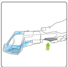
Start the unit then activate the trigger to circulate water around the cleaning head. Release the trigger and continue to run the unit until any excess water is cleared from the cleaning head and hose.
