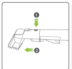
The cleaning head can be removed from the hose to clean.
