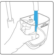
The water tanks can be rinsed with clean water. Use cold or warm water, maximum temperature 40°C
