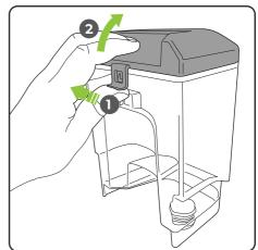
Pull the latch and remove the lid
