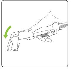
Tilt the cleaning head forwards and push firmly to the surface to collect excess water
