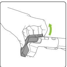
The front cover of the cleaning head can be removed to clean.
