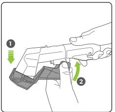
To fit the self-cleaning cover, hook the front of the cleaning head into the part then clip the back part to the handle.
