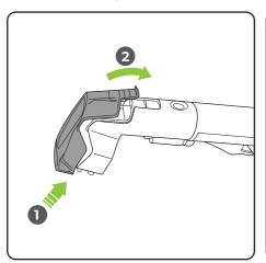
To re-fit the cover locate the bottom edge and then clip into place.
