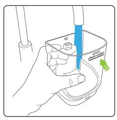
Add clean water. Do not fill above the level marked on the tank. Use cold or warm water, maximum temperature 40°C WARNING: do not use boiling water
