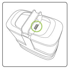
Replace the tank into the unit. Ensure the latch is located and the tank is securely engaged.
