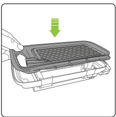
Fit the filter into the dust bin
