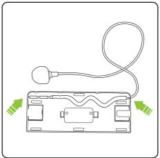
The charging stand cord is stored in the base. Pull the cord out to the required length, from either side of the unit.
