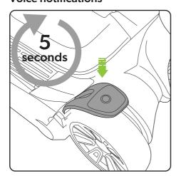
The voice notifications can be turned on and off. With the product switched off, press and hold the power button for 5 seconds to change the status.
