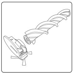
The brush bar can be removed from the end cap for more thorough cleaning
