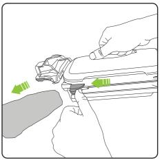
Hold the bin over a rubbish bin and slide the lever to open the bin door and empty the dirt.
