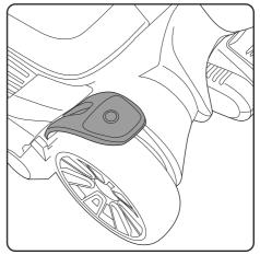
The power button is located on the left hand side of the head. Press the power button with your foot to turn the product on. Press the power button with your foot to turn the product off.
