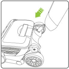
Locate the handle onto the steering pivot on the head.
