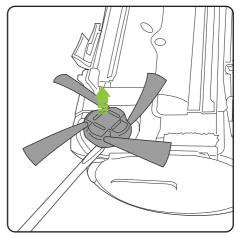
Carefully insert a small flat bladed screwdriver or similar tool into the gap around the edge brush.
