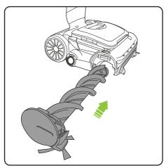
Push the brush bar into the product until it clicks into place. Check the brush bar is engaged onto the drive spindle.
