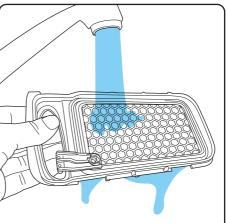
Wash the filter under a tap. Recommended water temperature 40°C. Do not use detergent or soaps. Let it dry completely before reinserting into the product.
