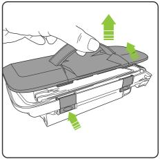
Press the 2 latches and lift off the bin lid
