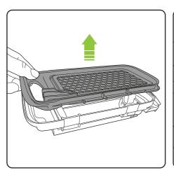
Remove the filter from the dust bin
