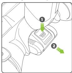
Press the release button and pull to remove the battery.
