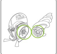
Note to assemble the matching end when re-fitting the brush bar to the end cap.
