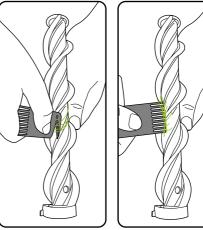
To remove hair from the brush bar, run the hair removal tool down the groove to cut the hair, then use the comb remove it.
