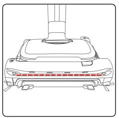
If the brush bar jams during use, the product will stop and the headlights will appear red. You will need to clean the brush bar and remove any blockage.
