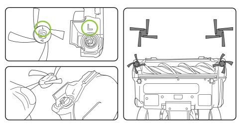
To re-fit align the brush onto the drive spindle and press the brush until it clicks into place. The edge brushes are handed and note to match the "L" and "R" markings on the brush and housing.
