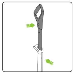
Should the upper handle need to be removed, press the button and use a suitable tool to press in the latch. Pull the handle upwards to remove.
