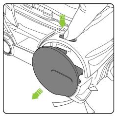
Before checking for a blockage, switch off and remove the battery. Press the button to release and eject the brush bar.
