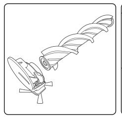
The brush bar can be removed from the end cap for more thorough cleaning
