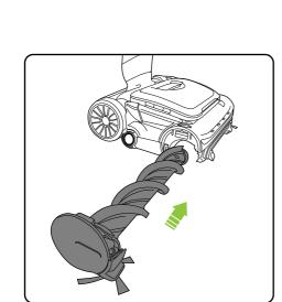
Push the brush bar into the product until it clicks into place. Check the brush bar is engaged onto the drive spindle.
