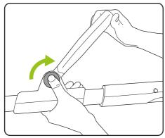
Push the button and rotate the handle to the required angle.
