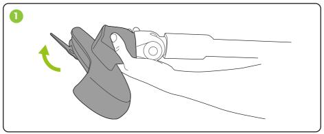
Firmly grip the main unit and rotate the head  $180^{\circ}$
