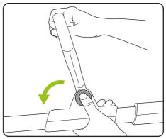
Release the button and ensure the handle clicks into a locked position.
