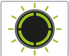
While charging the LEDs will progressively pulse until all four are lit.
