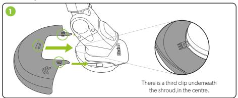
**Attach the shroud first.** Align all three clips on the shroud to the holes on the trimmer head and simultaneously push them into place. Once on, the shroud cannot be removed.
