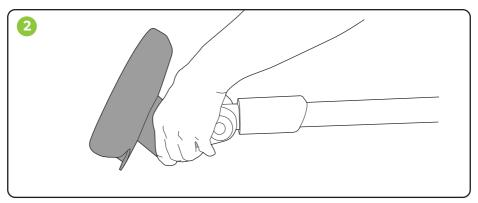
The head only rotates in one direction.
