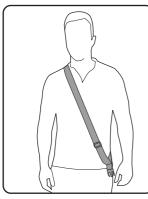
The harness is included as a safety feature for use with the branch cutter and the hedge trimmer. The sling passes over your head and rests on your shoulder - use the sliding adjuster to ensure the harness fits you comfortably.
