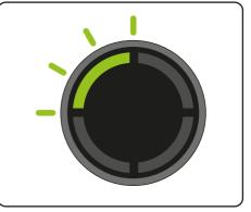
When there is no power left, the final LED will flash for 10 seconds then go out.
