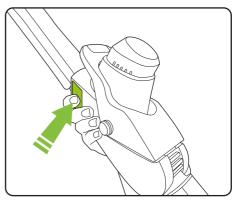
Press the green buttons on either side of the trimmer head.
