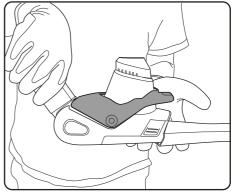
You can now rotate the head whilst pressing down on the lever. Release the lever and it will lock into place. This feature does NOT work with the branch-cutter.
