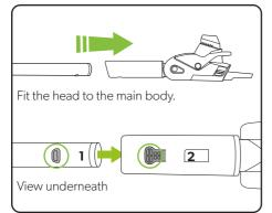
When the pole is fully inserted, the button (1) will pop up into the aperture (2). To remove, press the button (1) and pull the pole.
