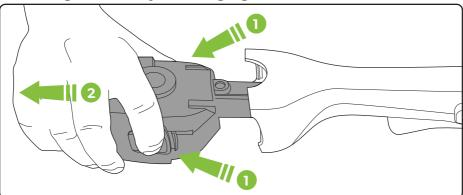
Removing the battery for charging
