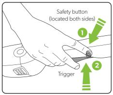
Push and hold the safety button on either side, then press the trigger to operate.
