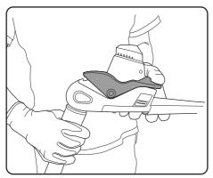
Remove the battery and ensure that the blade cover is on before continuing the next step. Depress the lever as shown. The head will now rotate freely.
