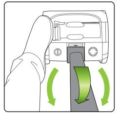
Without pressing the power button, place your foot on the left side of the AirRAM K9 head and pull the handle back.
