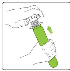
Slide the filter onto the inner shroud.
