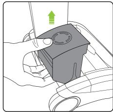
The battery can be charged whilst it's in the AirRAM, or when it's off the product. To remove the battery, squeeze the latch underneath and pull upwards.
