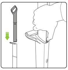
Insert the upper handle into the lower handle. You will need to press the button on the upper handle to fit it in.
