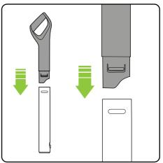
Fit the two components of the Upper Handle together in the orientation shown in the image above. They will only fit together one way. The components will click into place and will remain permanently fixed.
