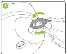
Hook a blade over the pin and pull to securely lock into place.
