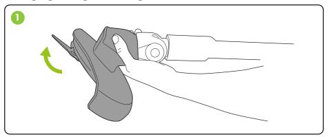
Firmly grip the main unit and rotate the head  $180^{\circ}$
