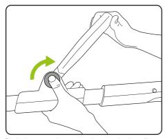
Push the green button and rotate the handle to the required angle.
