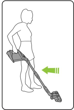
Pulling the vacuum back towards you activates the AirLOC and picks up finer particles.
