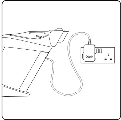
Plug the charger in and connect it to the charging port on the side of the battery.
