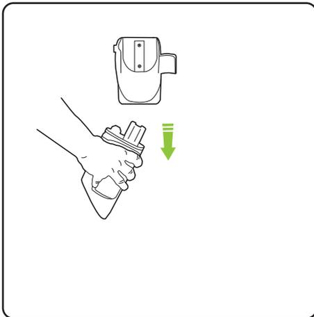
Pull the detachable tool kit out from the fixed section of the wall mount.
