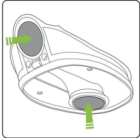
Remove the bag from the lid. Check for any blockages in the lid. Remove any blockages.
