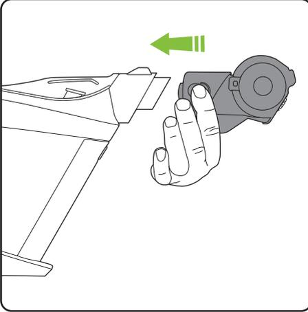
To attach the power brush, slot it over the standard nozzle. The power must be off while changing nozzles. The power button will now power the brush as well as the suction.
