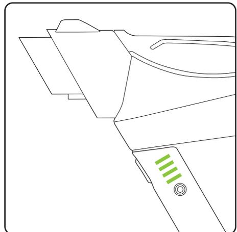
While the battery is on charge, the LEDs will pulsate and illuminate in turn. When the battery is fully charged, all of the LEDs will be solid green.
