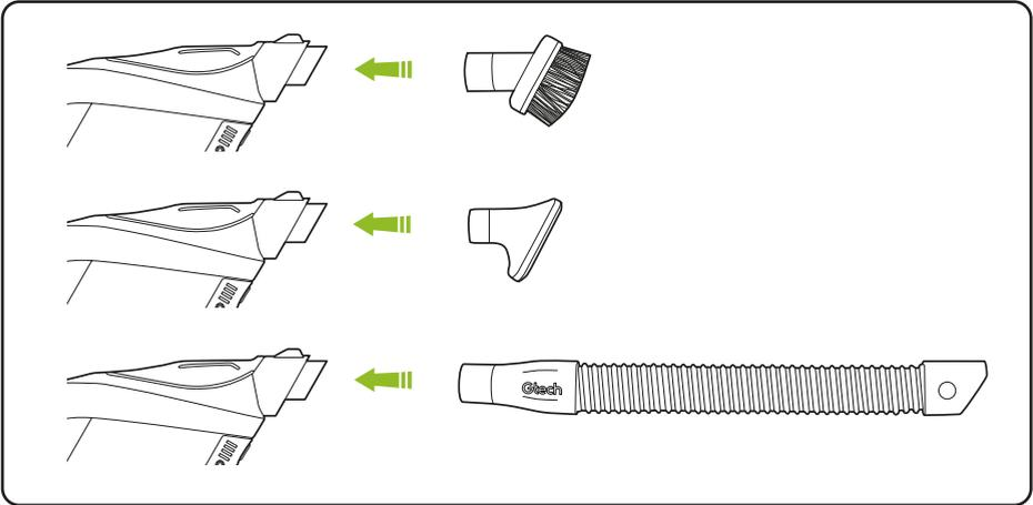
The three tools from the Car Accessory Kit fit directly into the nozzle of the product.
