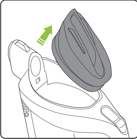
Remove the lid by pulling gently upwards.
