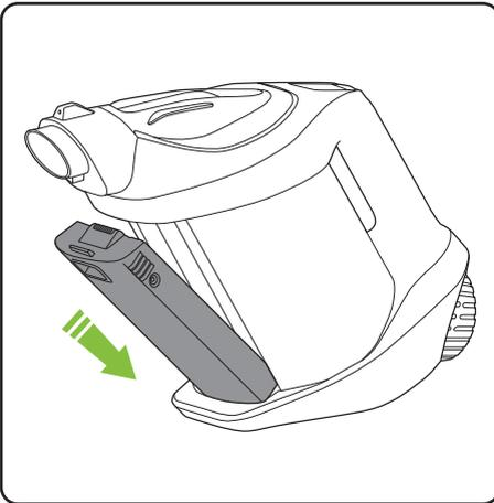
To replace the battery, slot it into the front of the product from the bottom first, with the latch facing outwards.
