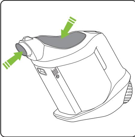
Remove the battery and lid and look through the nozzle. Remove any blockages.
