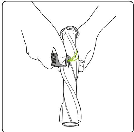
To remove hair from the brush bar, use the hair removal tool to cut the hair before pulling it out. Never operate the power floor head without the brush bar in place.
