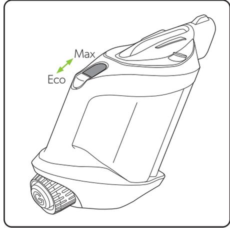
The product has 2 power settings: Max mode (higher suction power and shorter runtime) and Eco mode (lower suction power and longer runtime). Change modes by sliding the switch located in front of the On/Off button. The product will turn on in the mode it was last used.
