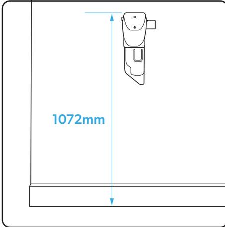
Install your wall mount at least 1072mm from the floor. Universal fixings have been included - please use the correct fixings for the wall type you're mounting this item to. Please use a stud finder to ensure no water pipes or electrical cables are hit. If you are unsure, please seek professional advice.
