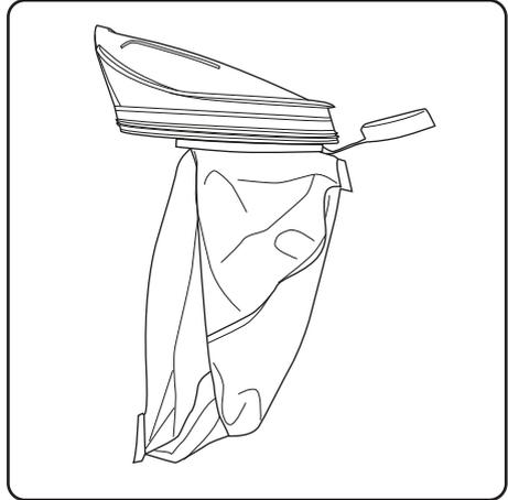
To get maximum efficiency from the bag, it is important to expand the bag before insertion.
