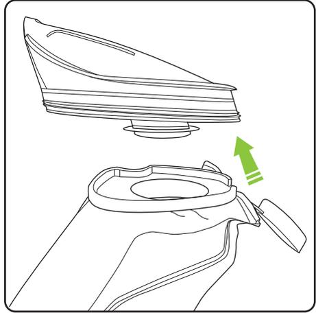
Fit the bag collar onto the tube underneath the lid and push it up firmly.
