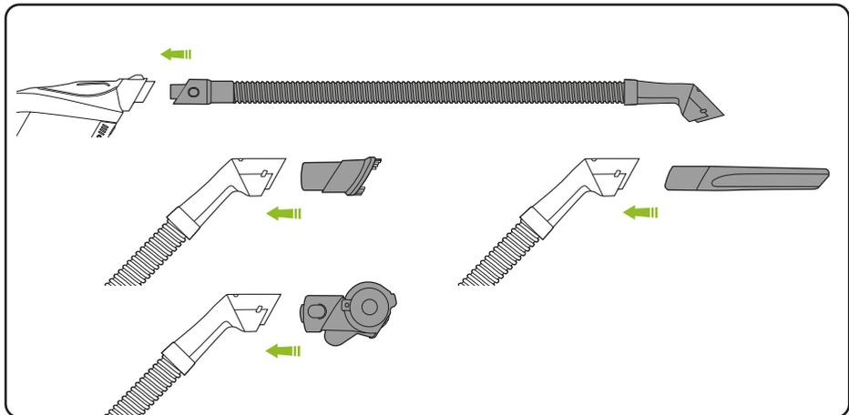
The flexible power hose attaches in the same way as the other accessories and can be used as it is or with the addition of other tools. Powered units can fit directly to the flexible power hose.
