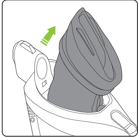
When the bag is full, lift the lid and remove it from the product with bag attached.
