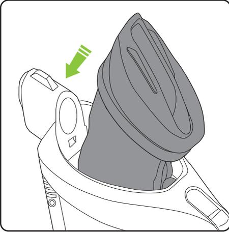
Once the bag is attached and straightened, place the lid back onto the main body, making sure the bag cap is also inserted.
