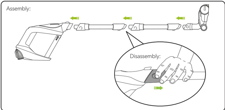
To use the product in floor cleaning mode, join the 2 sections of the extension tube and fit the power floor head at the end. Ensure all parts are correctly lined up and push them into place. Ensure the product is switched off before removing or fitting attachments. To disassemble, place your fingers in the indents of the tube, grip and pull the sections apart.
