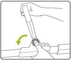
Release the button and ensure the handle clicks into a locked position.
