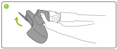
Firmly grip the main unit and rotate the head 180°
