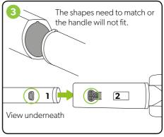
When the pole is fully inserted, the button (1) will pop up into the aperture (2)
