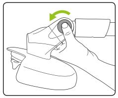
Push the button and rotate the head to the required angle.
