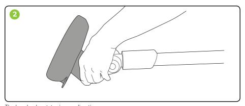
The head only rotates in one direction.
