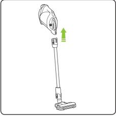
Attach the extension tube to the Gtech Pro K9.
