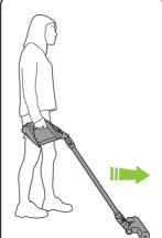
A forward motion will pick up Pulling the vacuum back larger pieces of debris. Pulling the vacuum back towards you activates the
