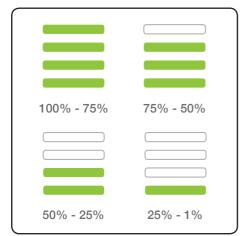
The battery state of charge indicator shows how much charge the Gtech Pro K9 has. As you use the product, the green lights will turn off in a downwards direction.
