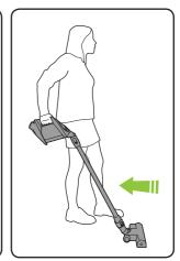
Pulling the vacuum back towards you activates the AirLOC and picks up fine particles.
