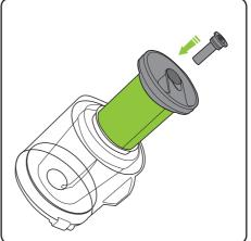
Place the new scented cartridge into the top of the filter.
