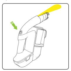
Press the button above the handle to turn the Power Floor K9 on and off.
