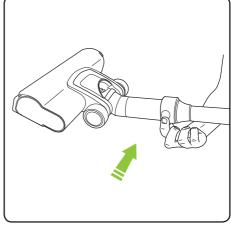
Before you remove the brush bar, you will need to remove the Power Floor K9 head from the extension tube. Gently pull on the green locking ring attached to the Power Head to remove.
