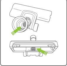
The Power Floor K9 head can also get blocked. To check for blockages thoroughly, remove the brush bar. (See page 9)
