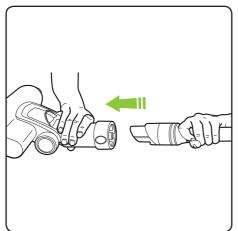
The power must be off while changing tools. Take the Power Floor K9 head and attach it to the extension tube.
