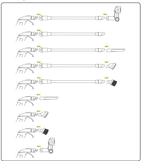
There are many configurations for the Power Floor K9. Refer to this diagram to see how each tool can be attached and used.
