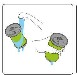
Wash the filter under a tap, squeeze it out then let it dry completely before using it. Use your spare filter while it dries. (You can get more at www.gtech.co.uk)
