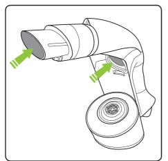
Remove the battery & bin from the body and look through both ends of the tube. Remove any blockages.
