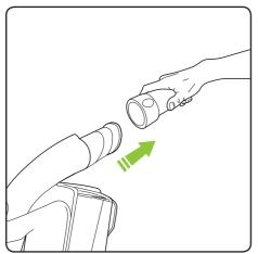
Remove the extension tube from the Power Floor K9 by pulling gently on the green locking ring.
