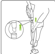
Attach the Power Floor K9 to the extension tube, making sure the white dots are aligned. The extension tube will click into place when correctly fitted
