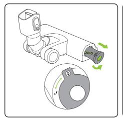
Before you remove the brush bar, you will need to remove the power floor head from the extension tube. Rotate the latch on the side of the powered floor head to the 'unlock' position and pull out the brush bar.
