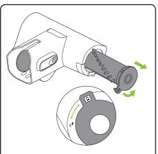
To clean the brush bar, first remove the power brush from the Gtech Pro. Rotate the latch from the lock to the unlock position and pull out to remove the brush bar.
