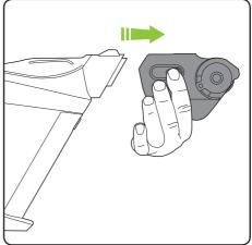
To remove the power brush, press the latches on the sides of the power brush and pull it away from the main unit.
