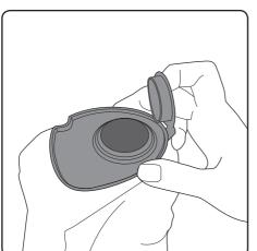
Carefully remove the bag from the Gtech Pro lid to avoid squashing contents. Insert the bag cap to secure contents.
