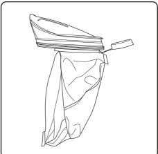
To get maximum efficiency from the bag it is important to expand the bag before insertion. Do not use the vacuum without a bag; it may damage the motor and will invalidate your warranty.
