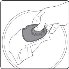
Dispose of the bag and replace with a new one.
