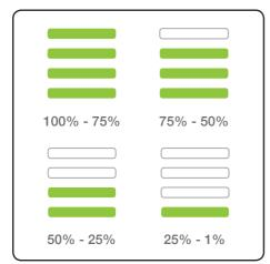
The battery state of charge indicator shows how much charge the Gtech Pro has. As you use the product, the green lights will turn off in a downwards direction.
