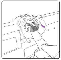
To assemble the lower handle Pull out the locking clip.
