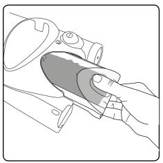
Remove the dust tray by pinching the window slightly, and pulling it out.
